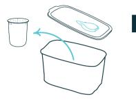
Remove reservoir from main body and remove cartridge from reservoir. Wash each component of the jug.
